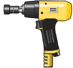
*For tools requiring high feed forces a high grip is preferred. For tools with only twisting forces, it is more important to have the handle in a forward position to reduce the wrist torque from the weight of the tool.*
