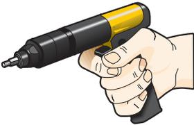
*On handles designed for high grip the trigger is operated with the middle finger while handles for the low grip have triggers operated with the index finger.*
