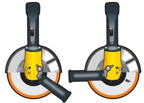
*Put the support handle in the most suitable position.*
