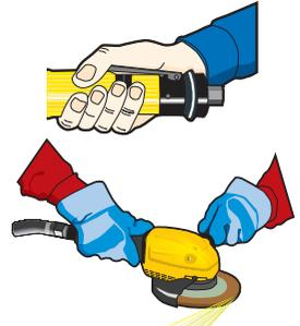
Angle nutrunners and rough grinders are normally equipped with a lever trigger.
