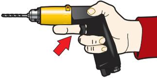
The drill handle designed for high push force has a high grip and a trigger operated with the middle finger.
