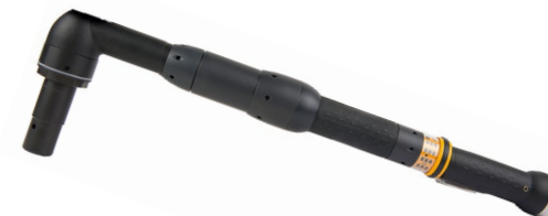
Example of assembled HAD for power tools
