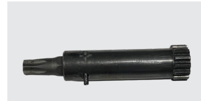
Locking with spring pin
